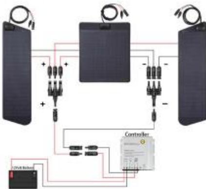
If you want to use the VSS panel to charge a power station, DO NOT connect the solar controller, just connect the solar panel leads to the power station. This is generally because most of the power stations available already come with a built-in solar controller.
