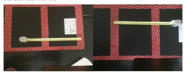
Use 2 rows of 1" wide 3M tape to align with each roof rib. Centre to centre spacing approximately 10 1/8"
