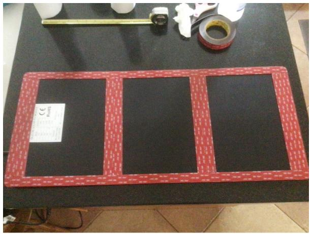
Clean the **Solar Panel** with alcohol before applying the 3M tape!!!
