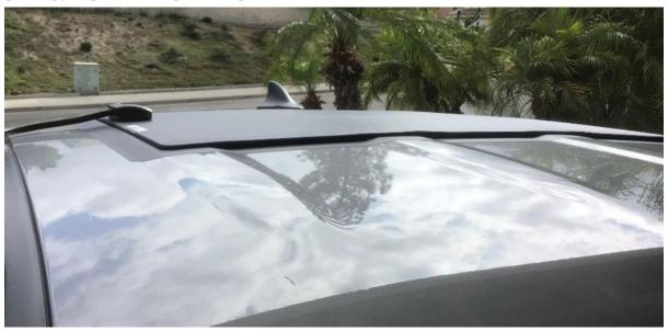
This **50W** solar panel is designed to fit the Gladiator JT. Its dimensions are 32.7×14". A larger panel will fit the top area of a **2014 Tacoma** Access cab. Use caution as the cab roof arch increases as it goes wider (front to back). A panel as wide as 28-29" may be possible but 21-22" would be a safer bet.
