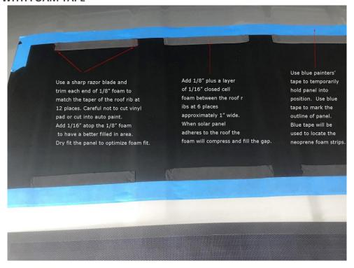
NOTE 1: Wash and then Clay bar roof area prior to installing the vinyl underlay. I used "Mothers Detailer"
