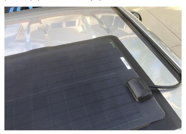
Vinyl Underlay was made larger than required in case the leading edge of the **roof solar panel** began to lift away at high speeds. The intent was to add Eternabond tape if this happened. 80-90MPH speeds and panel is still holding solid.
